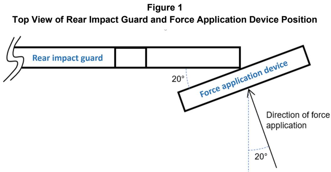
*Load application.* Apply the load in a direction that is perpendicular to the front surface of the load application device while guiding the device to prevent rotation. The loading rate should meet the CMVSS 223 criteria (section 5.3.1) and be applied until displacement of the force application device has reached 125 mm. The force should then be reduced until the guard no longer resists the force application device.
