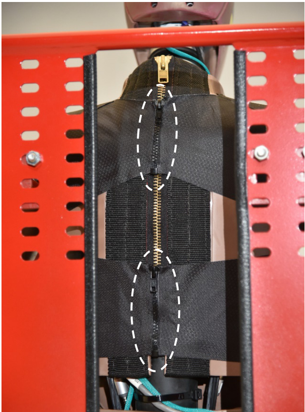
Figure A9. Securing the pressure sensor from the back
