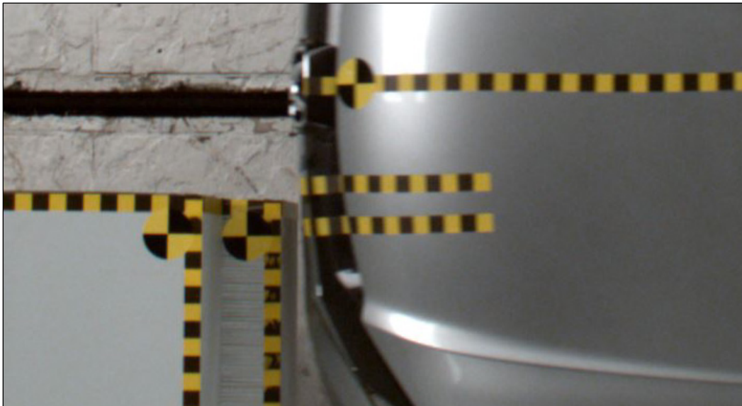
Figure 7 Determining vehicle overlap — Video screen shot
