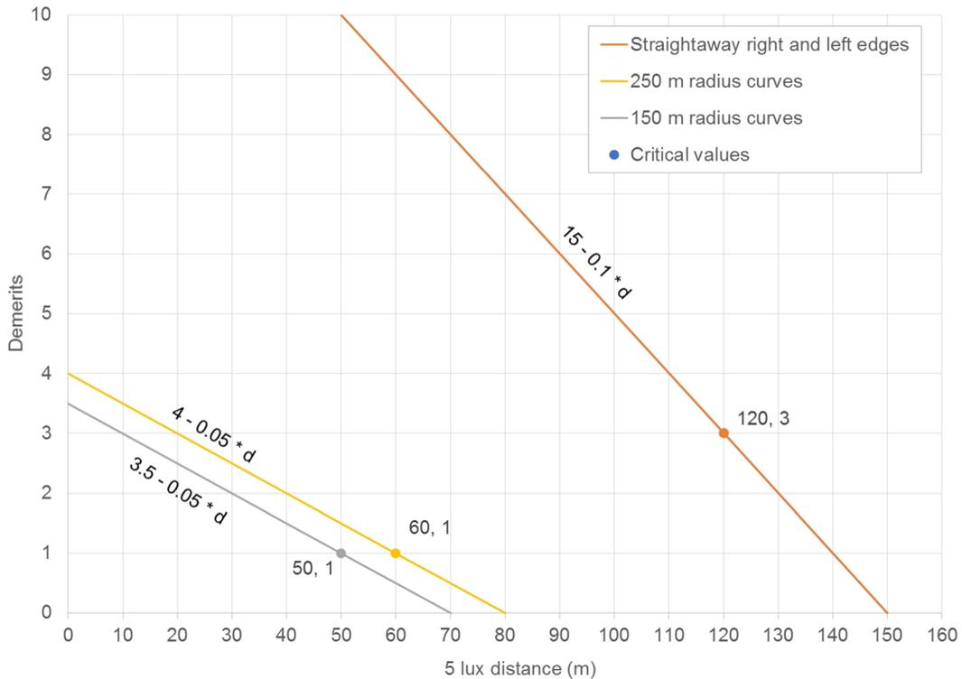
If the glare threshold was crossed for a specific low beam condition, the vehicle is assigned either the demerits in the “Critical value” column in Table 4 for that condition or the demerits calculated using the average 5 lux visibility distance, whichever is greater.
