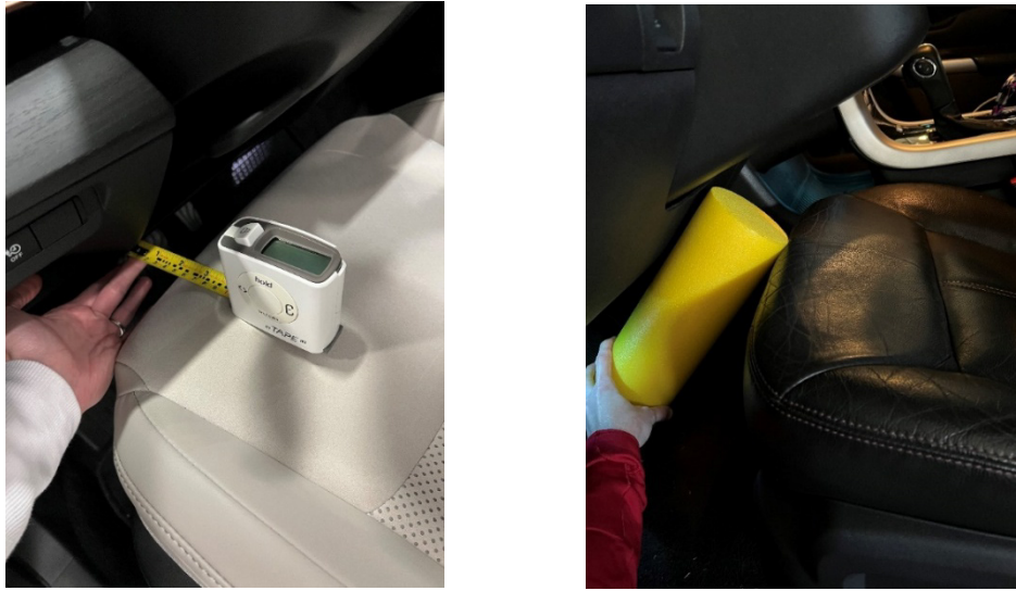
Figure 8 Foam roller check for the 5th-female's seating position (full forward and full up)
