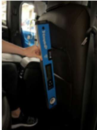
Figure 7 Large level for adjusting the driver seat back
