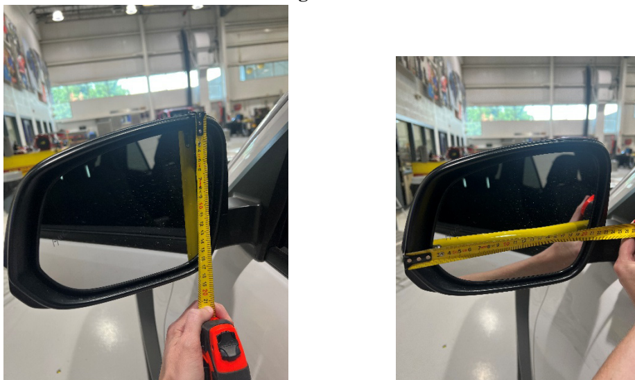
Figure 5 Measure the height and width of side mirror
