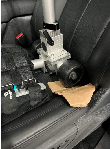
Figure 10 Example cardboard shim for leveling side-to-side
