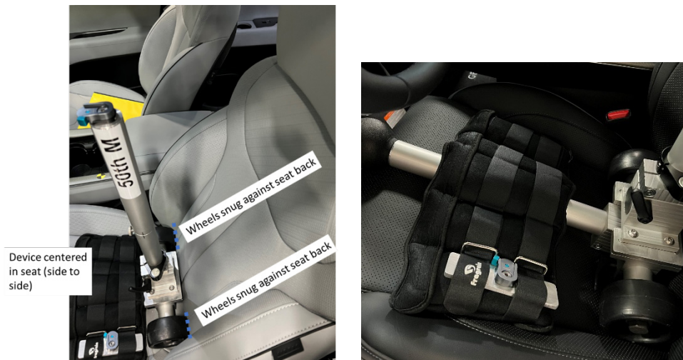
Figure 9 Adjust rig in driver seat and secure it
