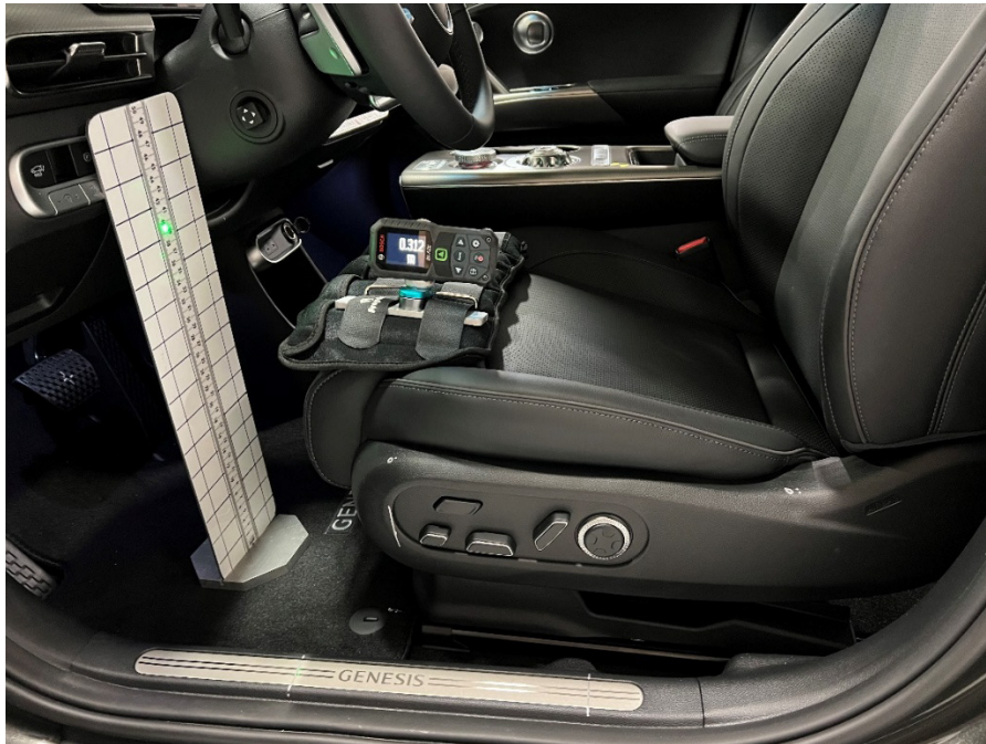
Figure 6 Digital measurement tool and floor target setup
