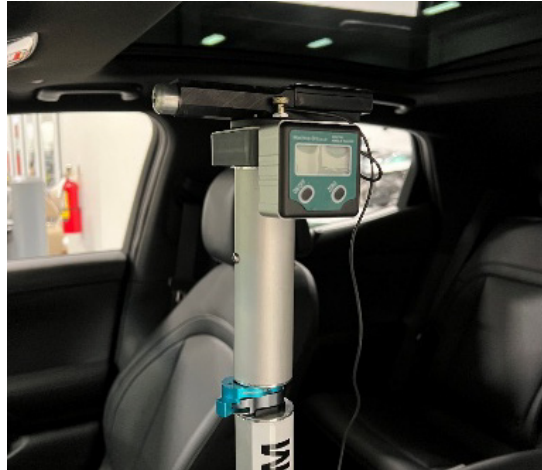
Figure 19 Laser angle tool attached to the rig
