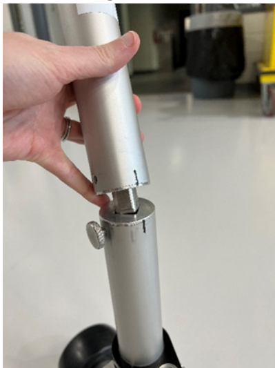
Figure 3 Align marks on neck extension and base and tighten set screw
