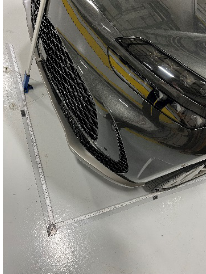
Figure 12 Coordinate system from foldable square: positioning the measurement pole
