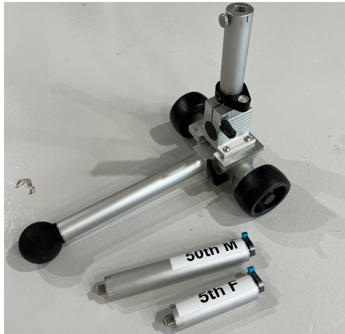
Figure 3 Align marks on neck extension and base and tighten set screw
