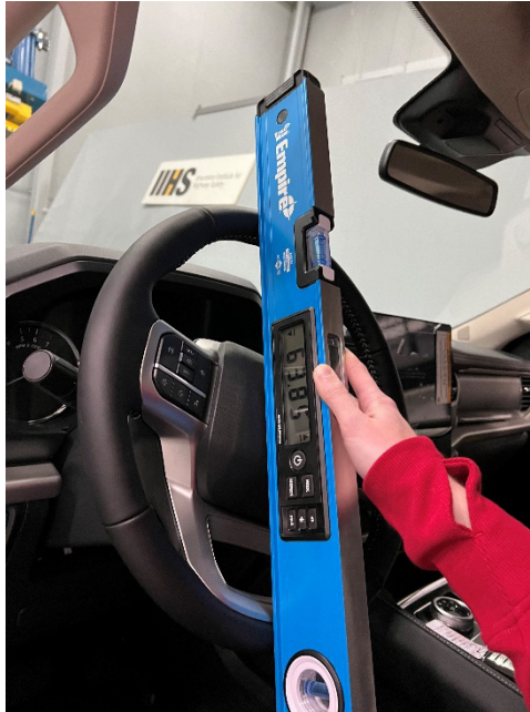
Figure 4 Large level to adjust the steering column's tilt angle
