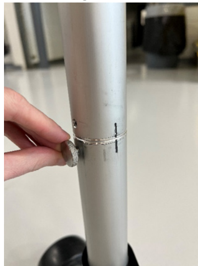
Figure 3 Align marks on neck extension and base and tighten set screw
