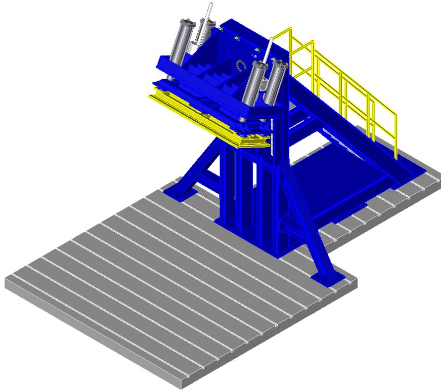
Two HR A-36 W10x88 I-beams are mounted on the bed plate perpendicular to the longitudinal axis of the platen. The vehicle, with attached rocker panel support system, is placed on these beams. The vehicle is adjusted so that:
