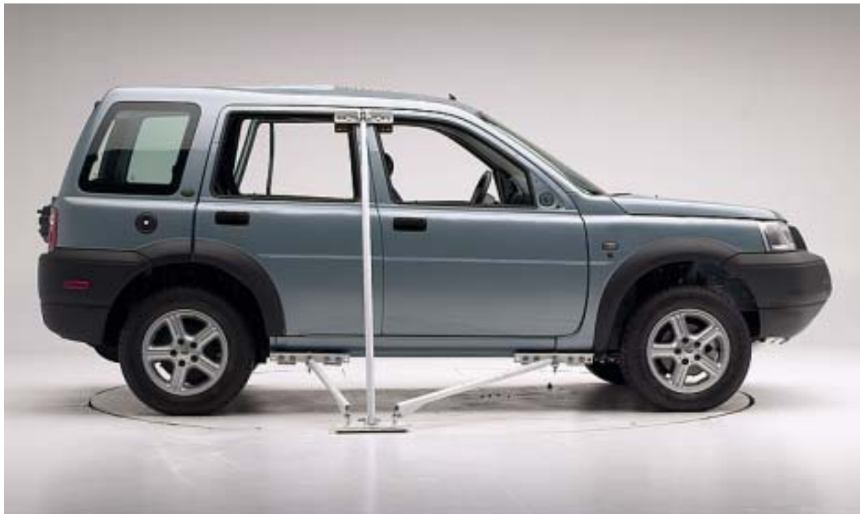
Figure 5 Antiroll Device for Tests of Sport Utility Vehicles, Pickups, and Passenger Vans
