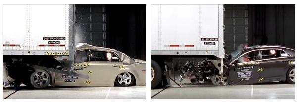
56 km/h, 50 percent overlap tests with 2007 Vanguard trailer (left) and 2011 Wabash trailer (right)
