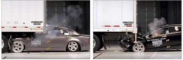
56 km/h, full-width tests with 2007 Hyundai trailer (left) and 2011 Wabash trailer (right)
