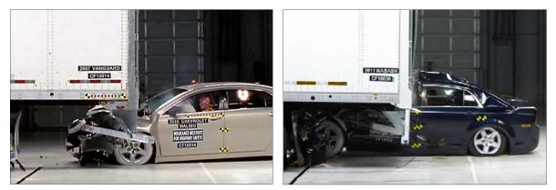
40 km/h, 50 percent overlap with 2007 Vanguard trailer (left) 56 km/h, 30 percent overlap test with 2011 Wabash trailer (right)
