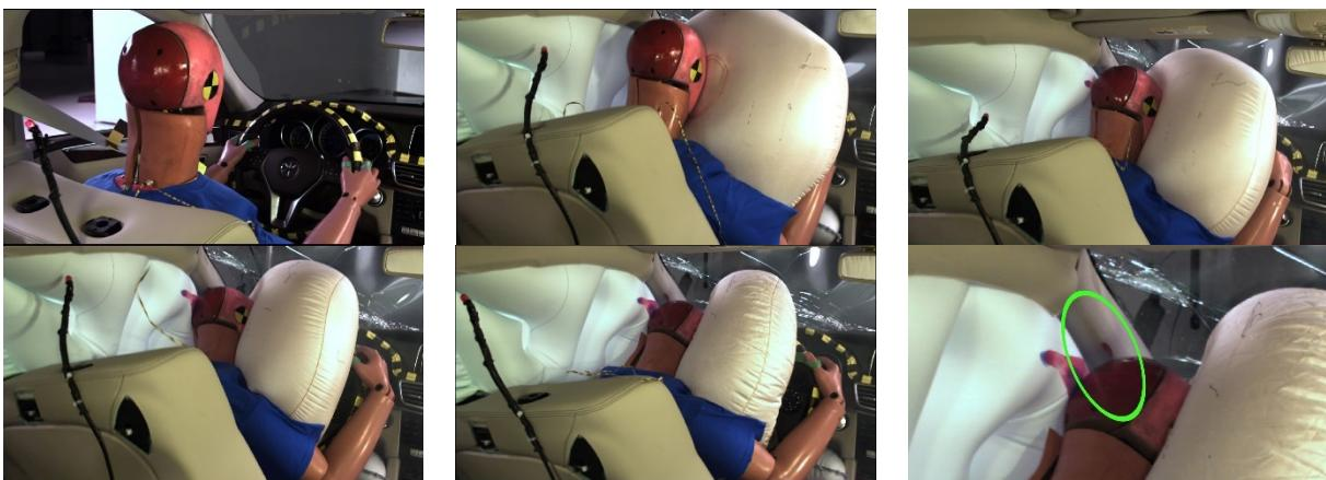
During the crash, the dummy's head loaded the frontal airbag but then rolled partly around it to the left side. The dummy's head contacted the a-pillar because there were no other countermeasures forward of the airbag.
