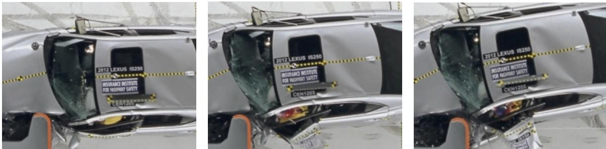
The outboard motion of the dummy, with respect to the vehicle interior, combined with the absence of a side head protection airbag allowed the most of the dummy's head to move outside of the precrash window plane.
