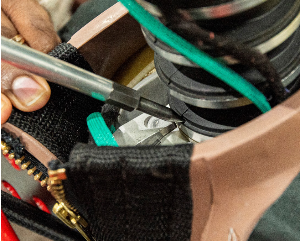
Figure A2 CMM point 2: Rear base of neck along dummy centerline
