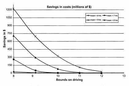
Fig. 6. Savings in cost for normal distribution (SD = 15% of mean).
