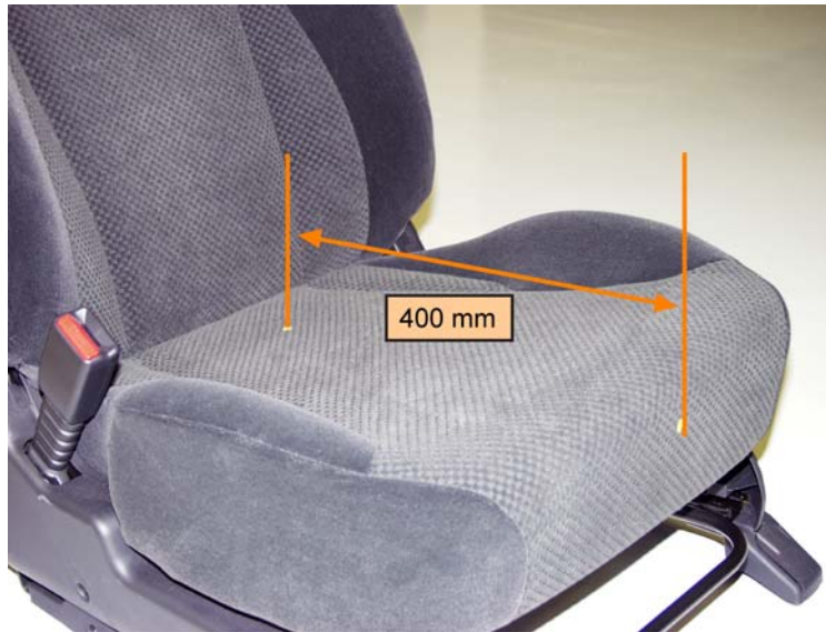
Figure 6 Seat Cushion Angle (400 mm measurement)
