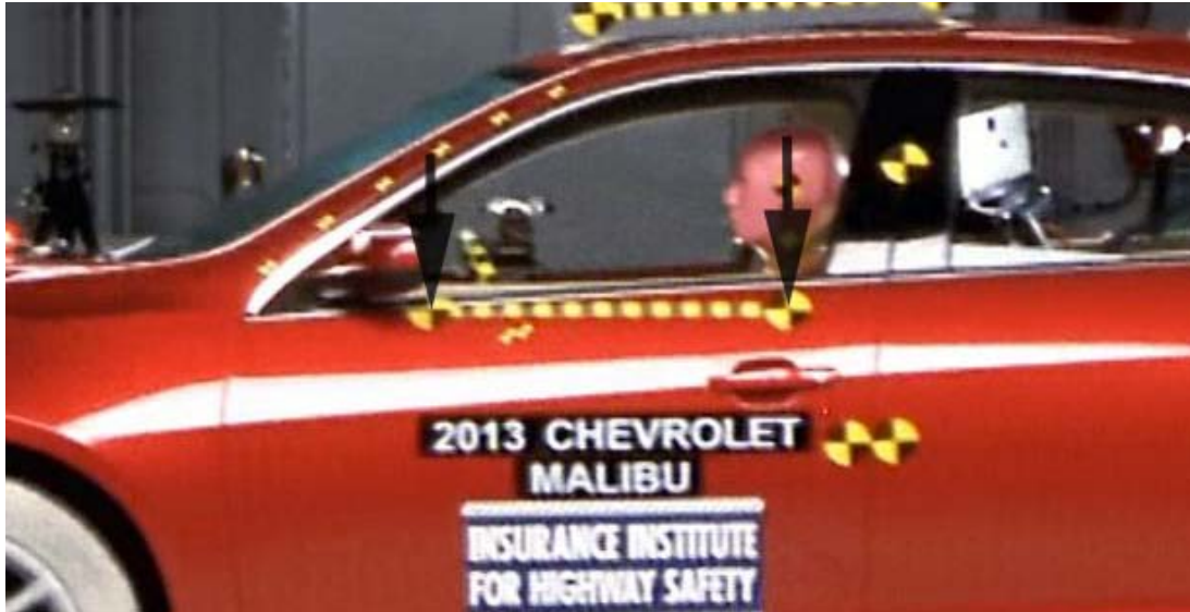
Figure A-2 Distance Between Horizontal Door Targets (61 cm), All Vehicles
