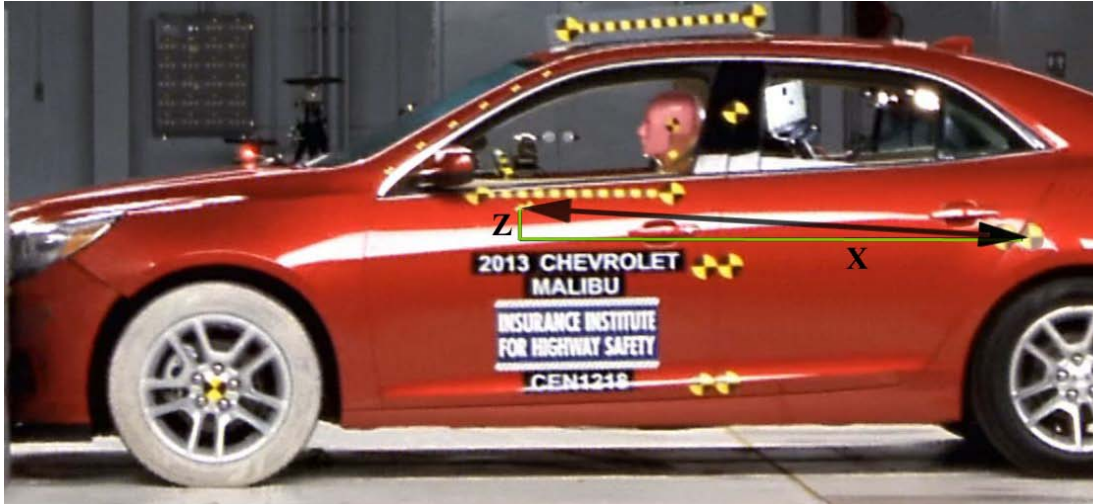
Figure A-1 Rear Door Latch Target to Steering Wheel Center Target Measure
