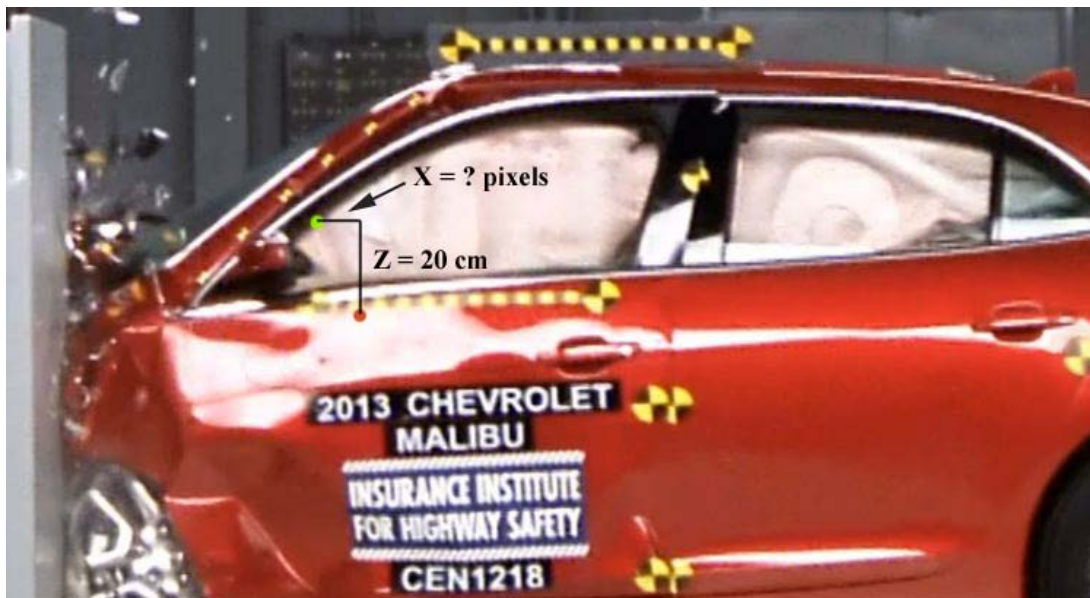
Figure A-4 Steering Wheel Center to Front of Side Curtain Airbag Chamber Measure
