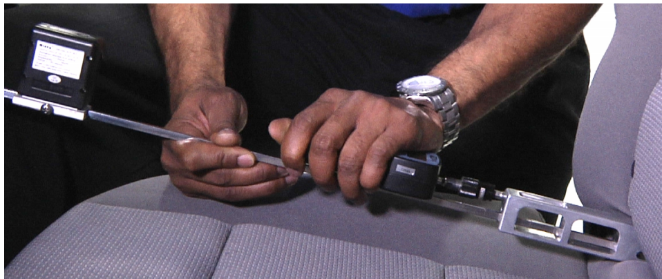
Figure 6. Measuring lower anchor attachment force.
