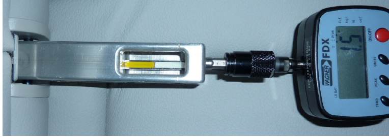
Figure 7. Force tool slider fully engaged on anchor.
