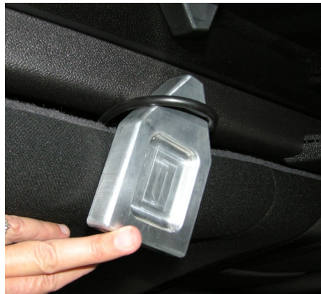
Figure 13. Bounded tether routing guide to route top tether strap between child restraint and tether anchor.
