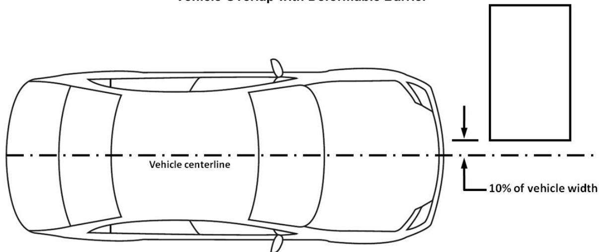
The vehicle is accelerated by the propulsion system at an average of 0.3 g until it reaches the test speed and then is released from the propulsion system 25 cm before the barrier. The onboard braking system, which applies the vehicle's service brakes on all four wheels, is activated 1.0 second after the vehicle is released from the propulsion system.
