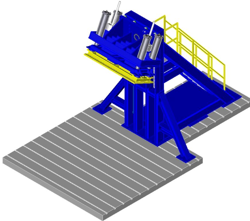
Two HR A-36 W10x88 I-beams are mounted on the bed plate perpendicular to the longitudinal axis of the platen. The vehicle, with attached rocker panel support system, is placed on these beams. The vehicle is adjusted so that:
