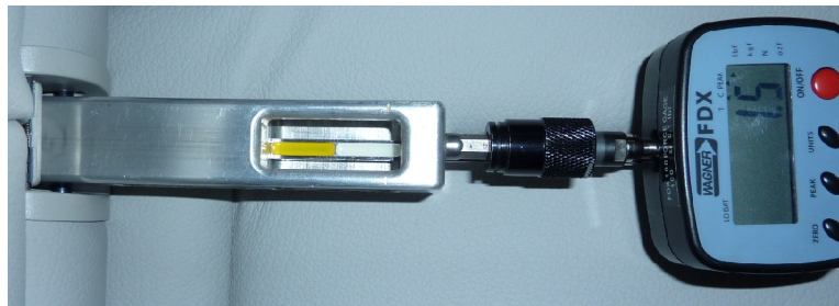
Figure 7. Force tool slider fully engaged on anchor.
