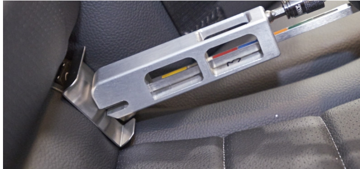
Figure 4. Initial position of force tool slider, with the tunnel adaptor just touching top and bottom of front surface of force tool slider.
