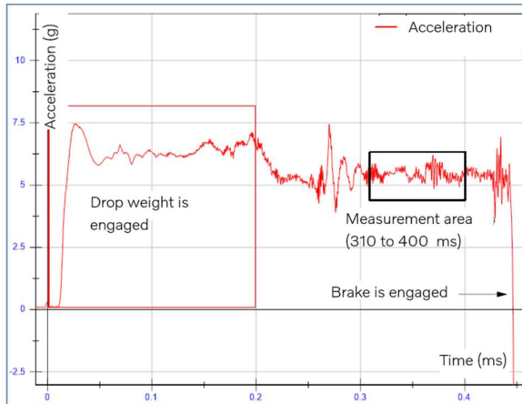
Figure 6 An example of the acceleration vs time, also indication what part is used for calculating the coefficient of friction.
