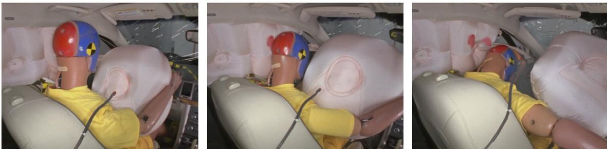
During the crash, the dummy's head missed the frontal airbag entirely, and there were no other countermeasures to prevent head contact with hard structures forward of the airbag.
