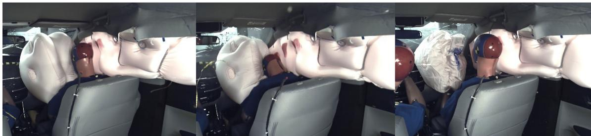
During the crash, the passenger dummy head loaded and remained engaged with the frontal airbag, with some additional help from the side curtain airbag.
