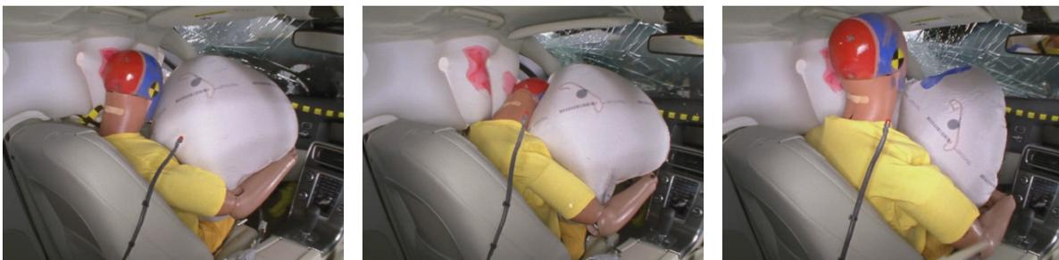
During the crash, the dummy's head briefly loaded the frontal airbag before sliding off the left into a gap between the frontal and side curtain airbags. The frontal airbag was narrow, and there were no other countermeasures to prevent head contact with hard structures forward of the airbag.
