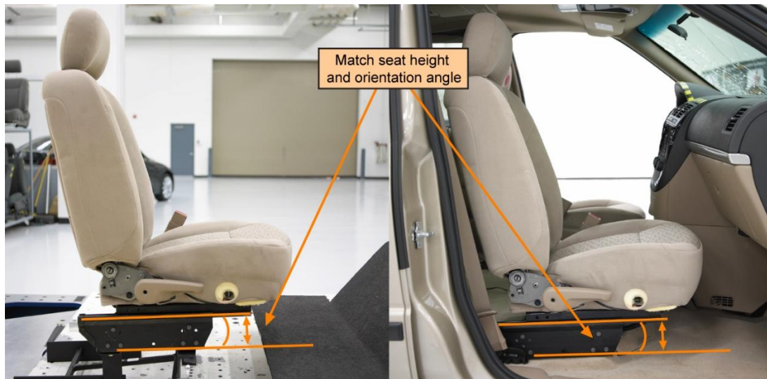
Figure 2 Attachment of seat to test sled compared with vehicle installation
