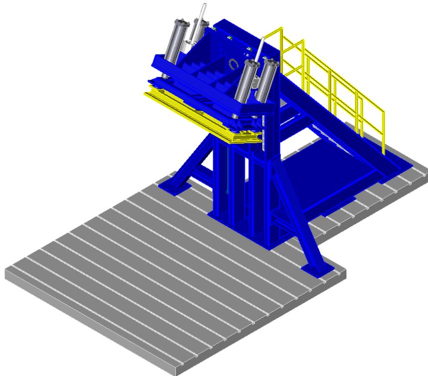
Two I-beams (HR A-36 W10x88) are mounted on the bed plate perpendicular to the longitudinal axis of the platen. The vehicle, with the attached rocker panel support system, is placed on these beams. The vehicle is adjusted so that:
