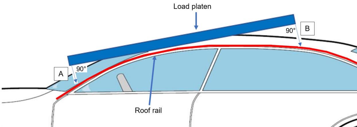
*Note:* The view shown is coplanar to the load face of the platen. The platen is positioned at the first point of contact. "A" indicates the front edge of the platen; "B" indicates the rear edge of the platen.
