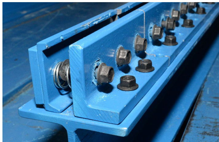
Figure 2 Rocker Panel Support System — Detail
