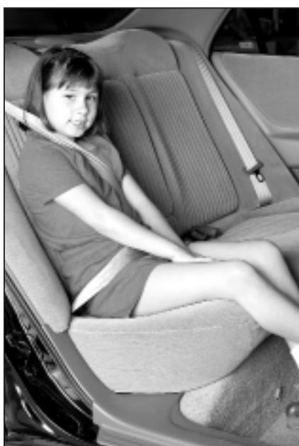
The main finding of this research is that booster seats enhance belt fit in some configurations. In others, a booster makes no difference or results in a poorer fit. All of this variability makes it difficult, if not impossible, to generalize about which groups of children would benefit from a booster seat requirement. It depends on the specific child, the specific booster seat, and the specific car model in which the two are positioned.
