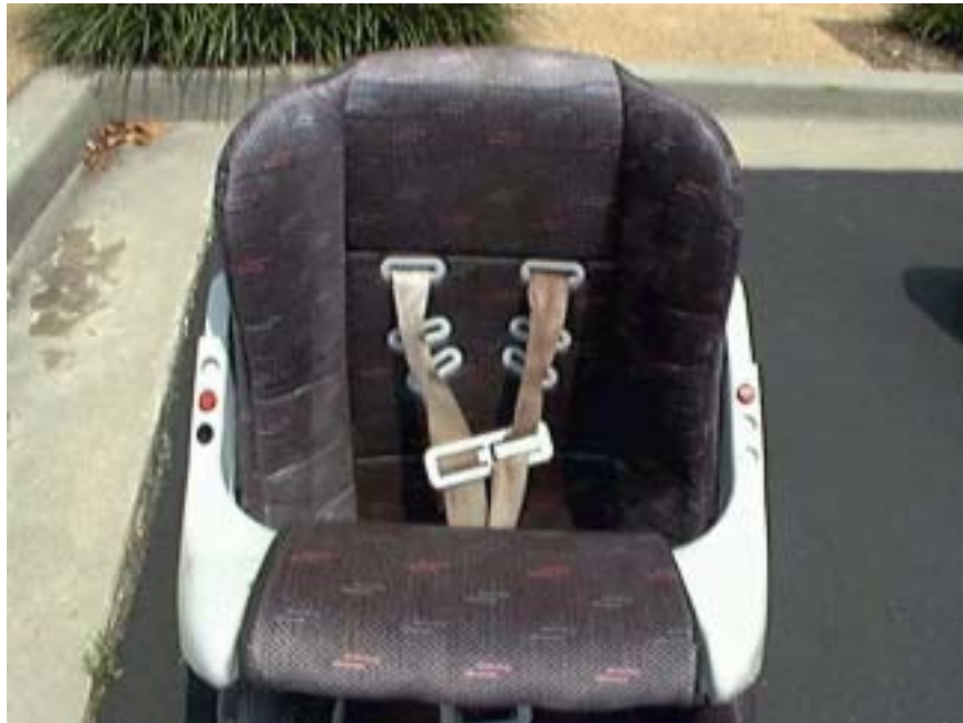
Figure 8 NASS/CDS Case PSU 1998-09-48K: Harness Misrouted in Top Slots Rather Than Middle Slots (From 1992 Ford Tempo Four-Door Car)
