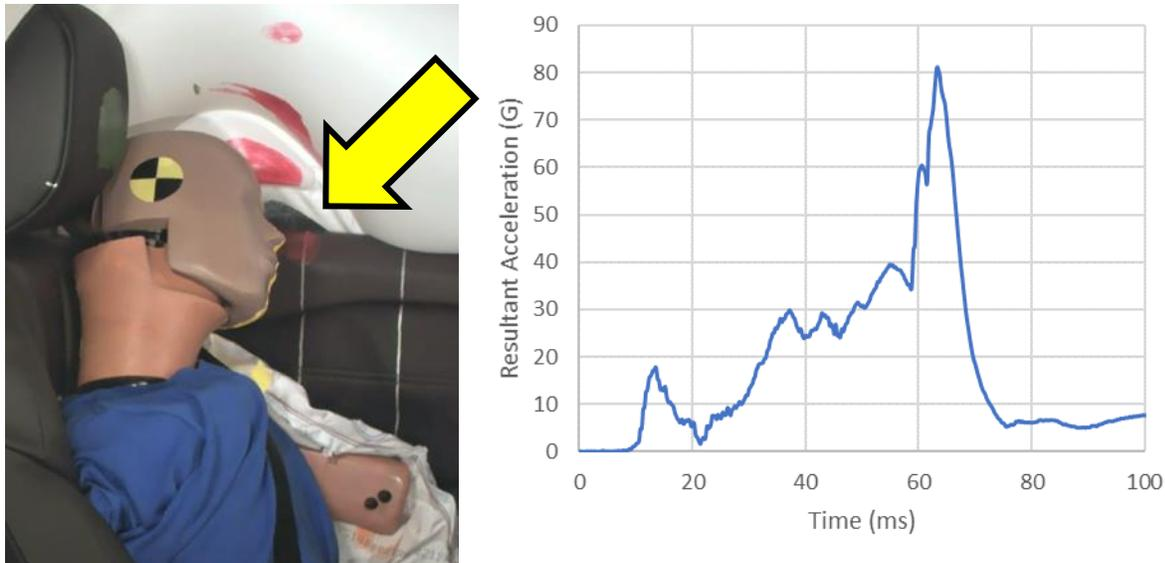
*Note:* The driver dummy's head contacts the door sill trim during the loading phase, with an associated resultant head acceleration peak of 80 G.
