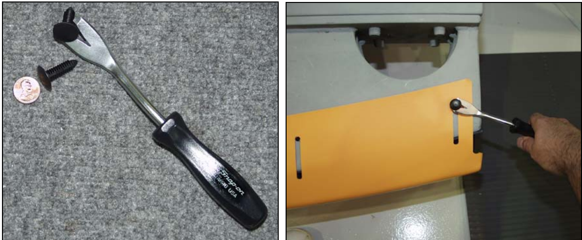
Figure 5 Nylon Push-Pin Rivet Fasteners (McMaster-Carr Part #90221A119)
