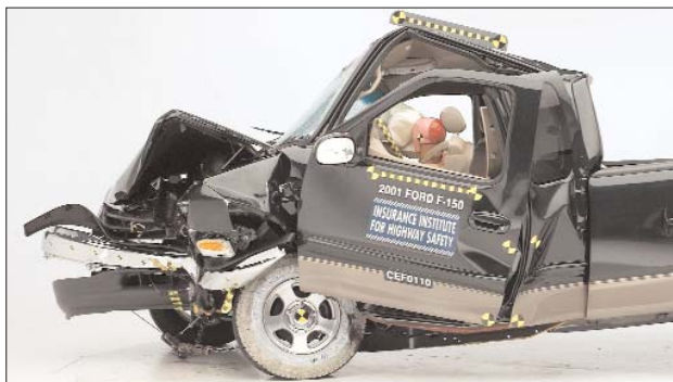
2001 FORD F-150 PICKUP Major collapse of the occupant compartment and roof deformation occurred in the Institute’s 40 mph frontal offset crash test.
