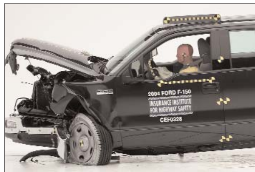
2004 FORD F-150 PICKUP Occupant compartment and roof remain intact in the Institute’s 40 mph frontal offset crash test.
