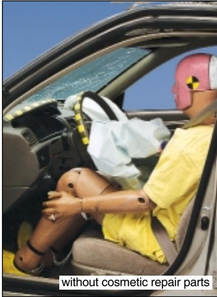
During each test, researchers recorded measures on the driver dummy to assess the likelihood that people in on-the-road crashes would be injured. These measures were similar. The dummy in the Camry without its cosmetic parts recorded slightly lower results for leg injuries, but the differences were well within the expected range of test-to-test variability.
