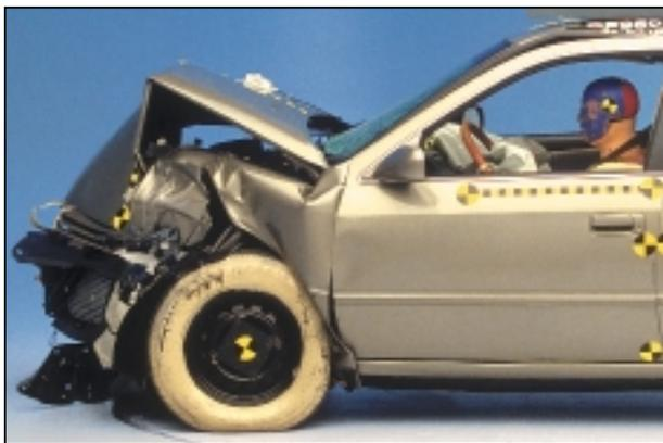
Both Camrys performed with distinction in 40 mph frontal offset impacts. Both earned good crashworthiness ratings according to the Institute's evaluation procedures. This means a Camry that does not have any of its front-end cosmetic parts is rated better than most competing midsize cars that still have such parts.
