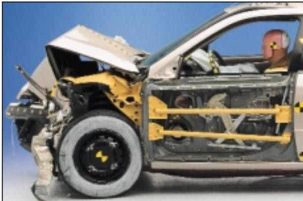
To demonstrate the irrelevance of safety in the cosmetic crash parts debate, the Institute recently tested a 1997 Toyota Camry from which the front fenders, door skins, and front bumper cover were removed (top photo). The original-equipment hood was replaced with a certified hood from an aftermarket supplier. The test results then were compared with results involving a 1997 Camry with its original-equipment parts intact (bottom photo).
