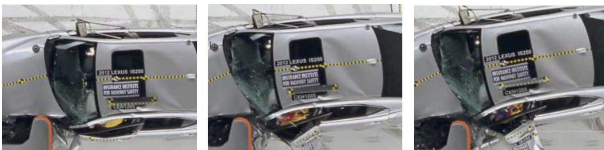
Figure 6 Example of Excessive Head Lateral Movement – Lexus IS 250 (CEN1205)
