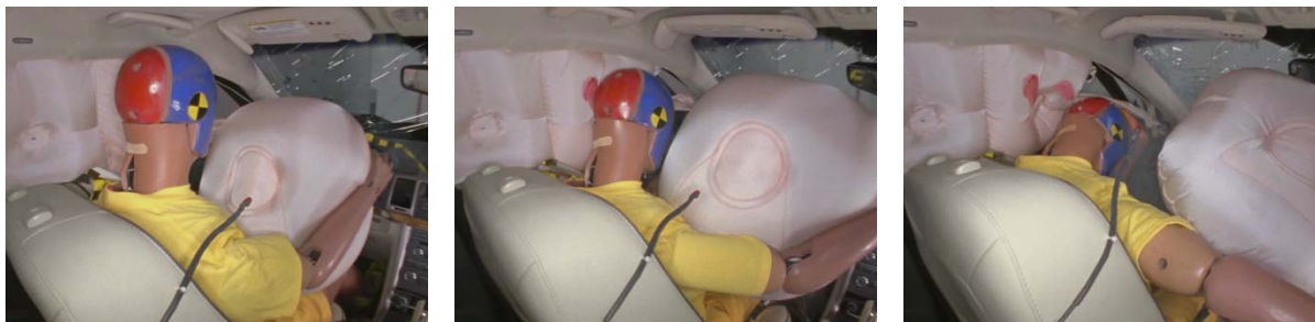
Figure 5 Example of Minimal Frontal Airbag Interaction – 2012 Lincoln MKZ (CEN1210)
