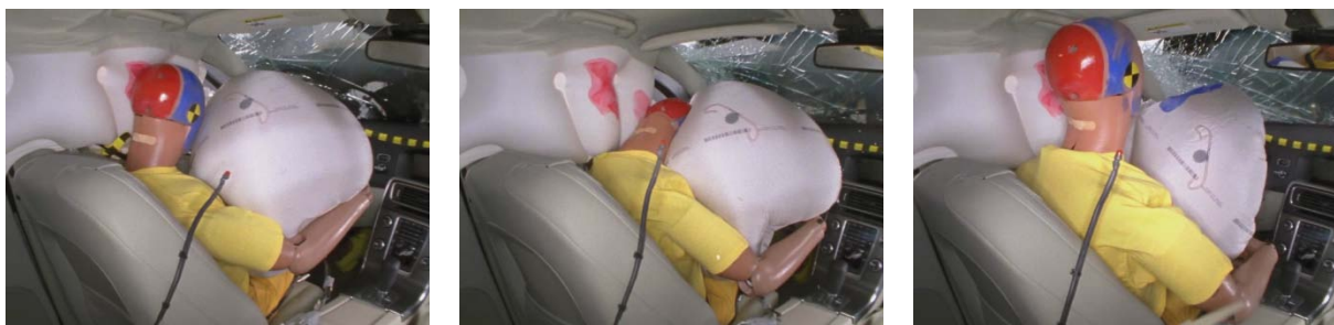
Figure 2 Example of Partial Frontal Airbag Interaction – 2012 Volvo S60 (CEN1207)
