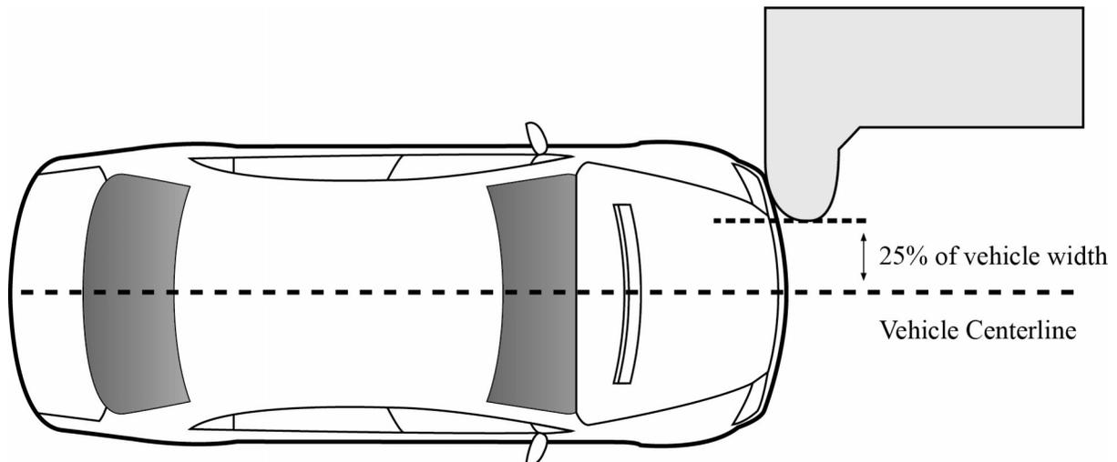
The vehicle is accelerated by the propulsion system at an average of 0.3 g until it reaches the test speed and then is released from the propulsion system approximately 25 cm before the barrier. The onboard braking system, which applies the vehicle's service brakes on the rear wheels, is activated 1.5 seconds after the vehicle is released from the propulsion system.
