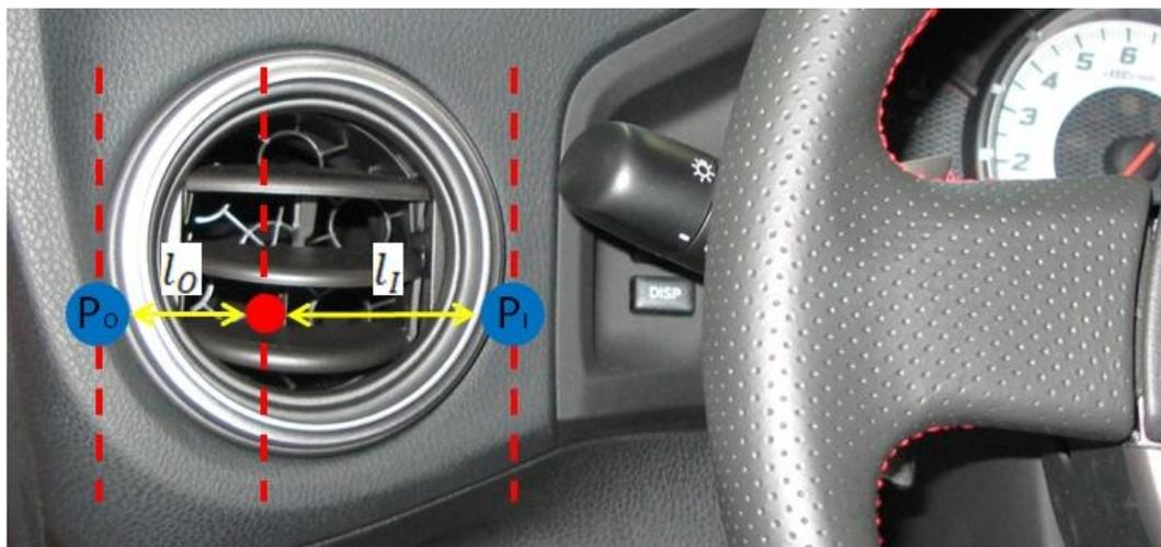
$$\text{Simulated upper dash point location} = \frac{l_I}{l_O+l_I} \times x_{P_O}, y_{P_O}, z_{P_O} + \frac{l_O}{l_O+l_I} \times x_{P_I}, y_{P_I}, z_{P_I} \quad (1)$$
