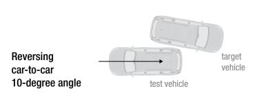
This scenario simulates backing toward the side of an adjacent stationary vehicle. The test involves reversing straight back toward the target vehicle parked at a 10-degree angle to the test vehicle.
