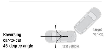
This scenario involves reversing out of a parking space toward a stationary vehicle. Test runs include reversing straight back and from the left and right toward the target. If autobrake fails to intervene, the corner of the test vehicle's bumper will strike the center of the target vehicle bumper.
