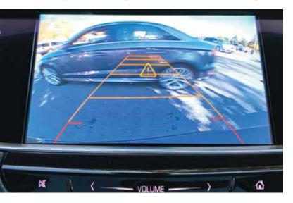
Parking sensors warn drivers if they get too close to another car or object behind or in front of them. Rear autobrake detects objects behind reversing vehicles and may brake if drivers don't heed alerts to stop. Rear cross-traffic alert warns backing drivers of approaching cars.
