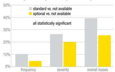
The frequency of glass claims for Kia SUVs with standard panoramic roofs was 10 percent higher than for Kia models without available panoramic roofs. Glass claim severity was 26 percent higher, and overall losses were 39 percent higher for Kias with standard panoramic roofs versus the same SUVs without them.
