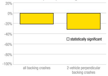
(*« from p. 5)* The GM models studied could have had a rearview camera alone; parking sensors alone; rearview camera plus parking sensors; rear autobrake, rearview camera and parking sensors; or none of these features. Rear autobrake was only available on the Cadillacs. The study controlled for the presence of rear cross-traffic alert, which was on some vehicles with both the rearview camera and sensors and all vehicles with rear autobrake.
