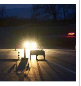
IIHS engineers test headlights at night on the outdoor track at the Vehicle Research Center in Ruckersville, Va.
