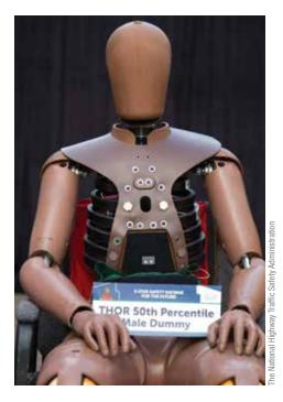
The THOR 50th percentile male dummy would replace the Hybrid III dummy in NCAP tests under NHTSA's proposal.
