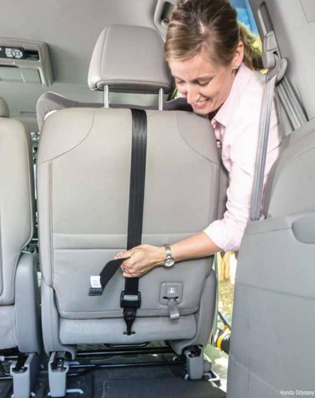
Tether anchors should be easy to find on the rear deck in sedans or the top 85 percent of the seatback in minivans and SUVs. In the above photo, the tether anchor is hard to find because it is too close to the bottom of the seat. Some vehicles have hardware such as cargo hooks that could be confused for the anchor. In that case, the tether anchor should be clearly labeled.
