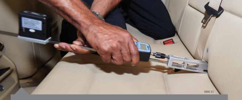
**How lower anchors are evaluated**: An IIHS engineer uses a specialized tool (above) to measure the depth and required force of a lower anchor. Another tool (below right) is used to measure the anchor's clearance angle. The Ford Edge is an example of a vehicle with anchors that are at the surface and clearly visible. In contrast, the Acura RDX's anchors are too deep within the seat.
