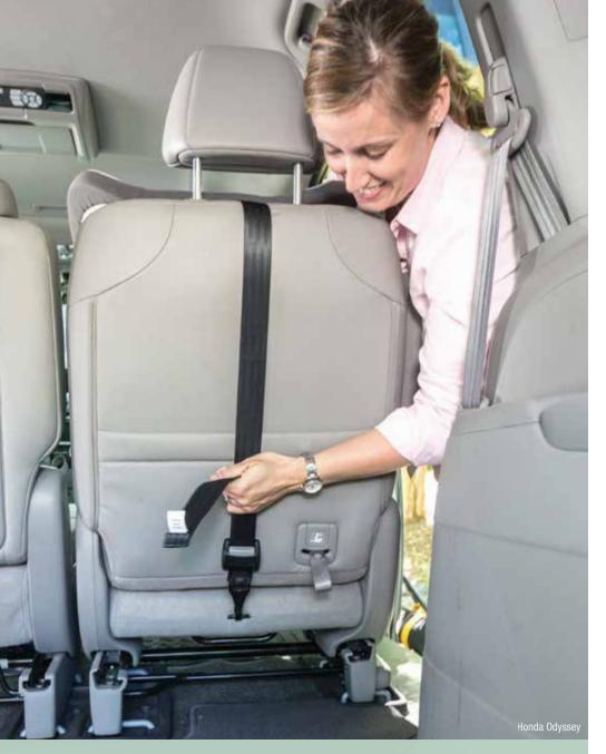
Tether anchors should be easy to find on the rear deck in sedans or the top 85 percent of the seatback in minivans and SUVs. In the above photo, the tether anchor is hard to find because it is too close to the bottom of the seat. Some vehicles have hardware such as cargo hooks that could be confused for the anchor. In that case, the tether anchor should be clearly labeled.
