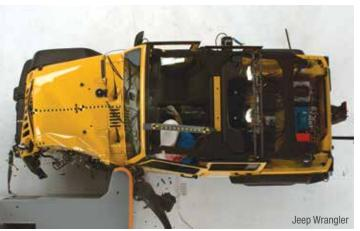
The Jeep Wrangler deflected off the barrier, which limited the forces on the vehicle, resulting in a good rating.
