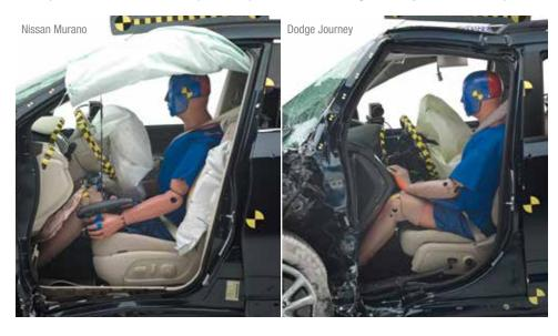
maximum intrusion of 4 inches in the left footwell. Forces on both of the dummy's lower legs were just high enough to indicate a moderate risk of injury in a crash of this severity.
