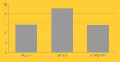
For calling a contact, the embedded vehicle systems reduced total eyes-off-the-road time compared with manual calling more than the smartphone voice interface. For entering an address, Volvo's Sensus system required the most time looking away but made few errors.
