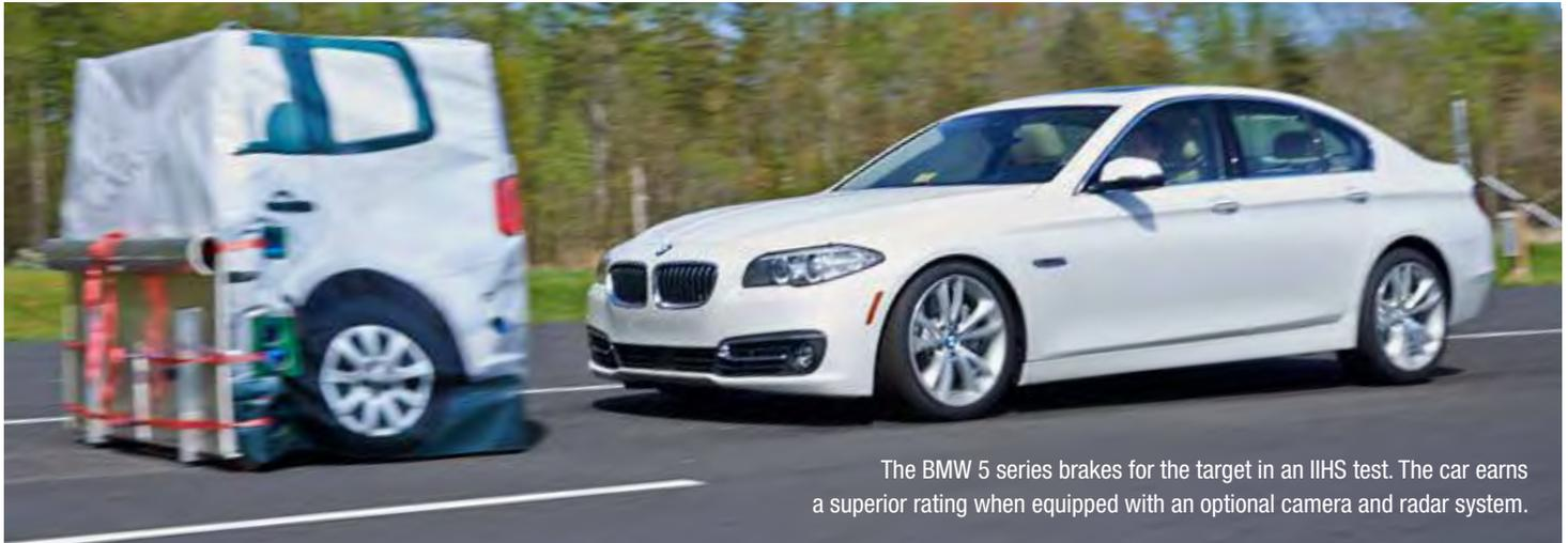
The BMW 5 series brakes for the target in an IIHS test. The car earns a superior rating when equipped with an optional camera and radar system.
