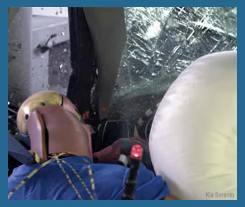
Five midsize SUVs received a poor rating for structure, the most fundamental aspect of occupant protection. In five vehicles, the dummy's head barely contacted the frontal airbag before sliding off.
