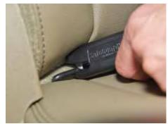
Attachment anchors that are easy to find and access raise the chances that parents will correctly use LATCH to install a child restraint. correctly install child restraints using LATCH, and the reason why depends a lot on the location and ease of use of attachment hardware in vehicles. A new IIHS study conducted with the help of Safe Kids Worldwide reinforces prior work indicating that modifying LATCH anchor setups in vehicles could improve child restraint installation rates.
