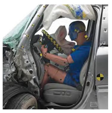
Survival space: The structure of the Chevrolet Equinox (left) held up well, leaving adequate space for the driver. In contrast, the driver space in the Honda Pilot was seriously compromised. In the worst instance of intrusion, the parking brake pedal moved inward more than 16 inches.
