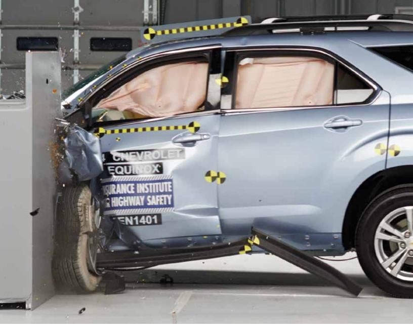
he Chevrolet Equinox and its twin, the GMC Terrain, are the only midsize SUVs out of nine evaluated to earn a good rating in the IIHS small overlap front crash test, which continues to challenge manufacturers more than a year and a half after its introduction.
