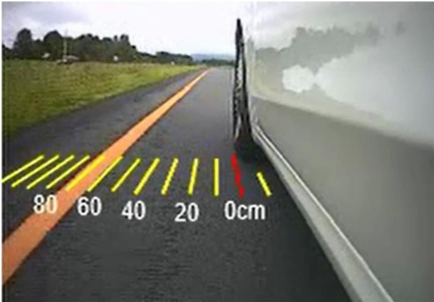
**Figure 1.** View from driver-side outboard camera on rear door. Ruler overlay was used to estimate distance (cm) from vehicle to lane marker.
