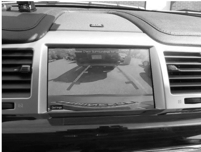
**Figure 1. Rearview camera image in the center console display**
