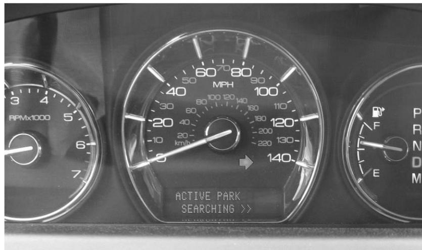
**Figure 2. Two-line text display with Active Park Assist system status and instructions**
