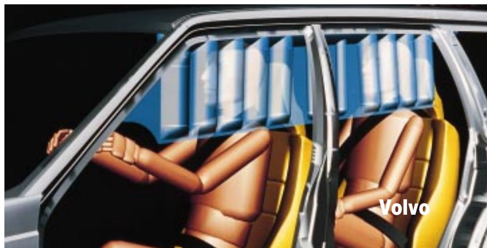
Mercedes and Volvo as well as BMW are equipping some models with head protection systems that inflate from the roof. Saab and Ford have airbags that protect people's heads in side impacts, too, but because these airbags don't deploy from the roof, they're unaffected by the rule change.
