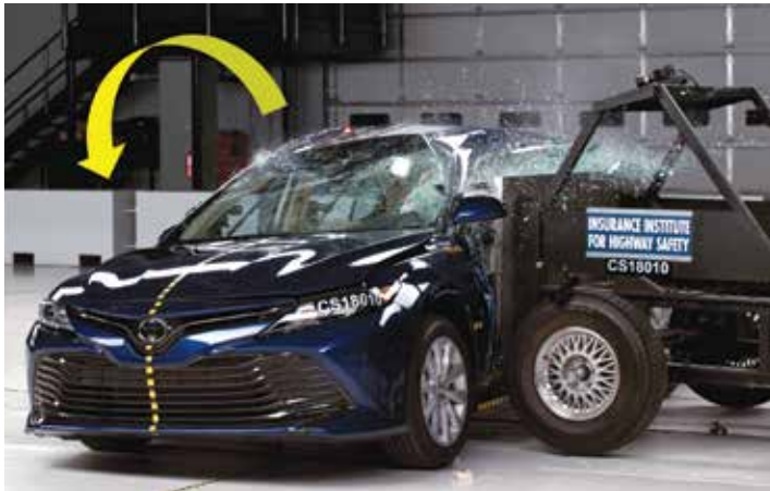
Movable barrier: Test vehicle rolls away from striking barrier
