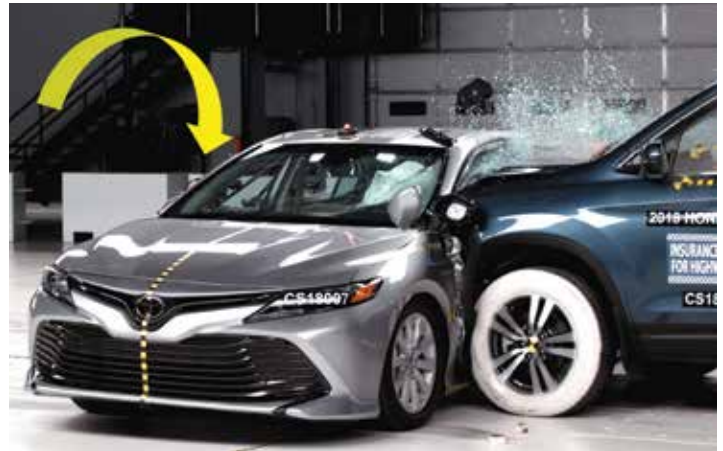
SUV: Test vehicle rolls toward striking SUV
