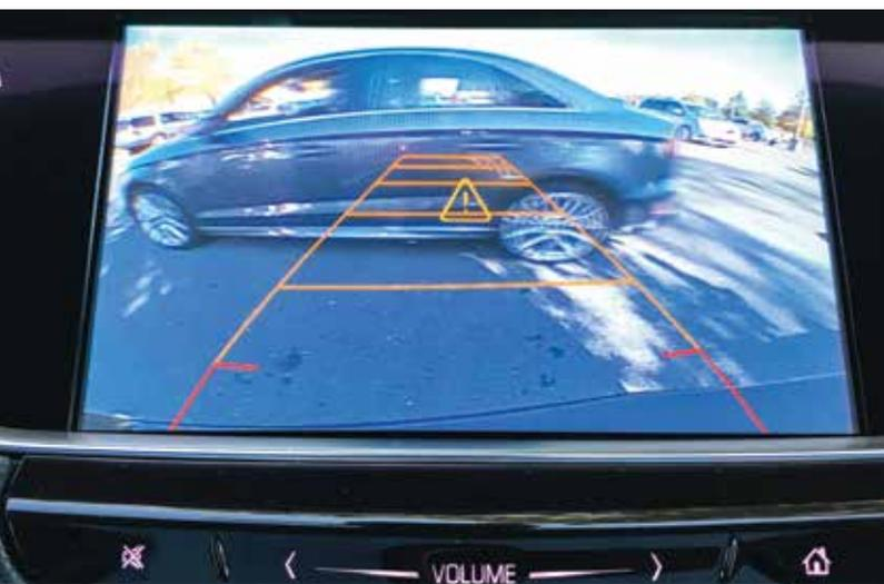
Parking sensors warn drivers if they get too close to another car or object behind or in front of them. Rear autobrake detects objects behind reversing vehicles and may brake if drivers don't heed alerts to stop. Rear cross-traffic alert warns backing drivers of approaching cars.
