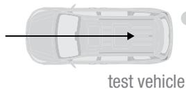
This scenario simulates backing into a pole or garage pillar. The test car reverses straight toward a bollard that is aligned midway between the center line and bumper corner.
