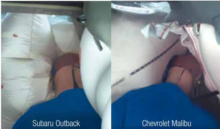
In the passenger-side small overlap test of the Subaru Outback (left), the passenger dummy's head hit the front airbag and stayed there until rebound. In the Chevrolet Malibu's test (right), the passenger dummy's head went between the front and side curtain airbags and hit the dashboard.
