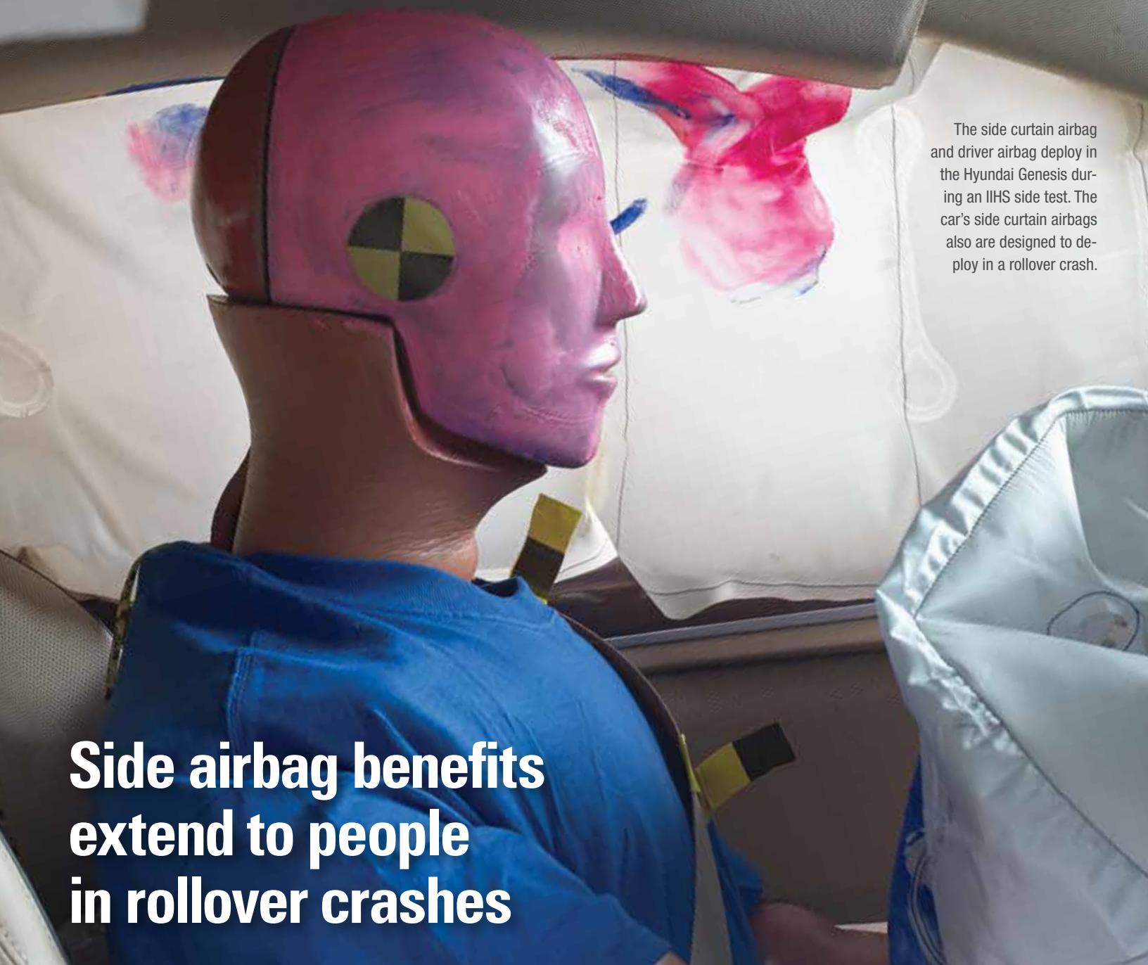
The side curtain airbag and driver airbag deploy in the Hyundai Genesis during an IIHS side test. The car's side curtain airbags also are designed to deploy in a rollover crash.
