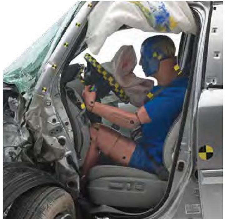
**Survival space:** The structure of the Chevrolet Equinox (left) held up well, leaving adequate space for the driver. In contrast, the driver space in the Honda Pilot was seriously compromised. In the worst instance of intrusion, the parking brake pedal moved inward more than 16 inches.
