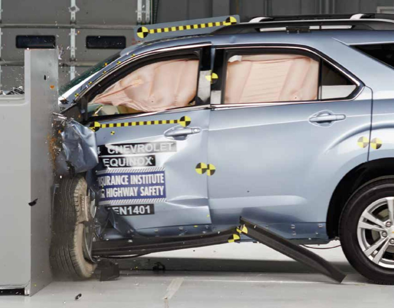
The Chevrolet Equinox and its twin, the GMC Terrain, are the only midsize SUVs out of nine evaluated to earn a good rating in the IIHS small overlap front crash test, which continues to challenge manufacturers more than a year and a half after its introduction.
