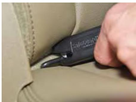
Attachment anchors that are easy to find and access raise the chances that parents will correctly use LATCH to install a child restraint.
