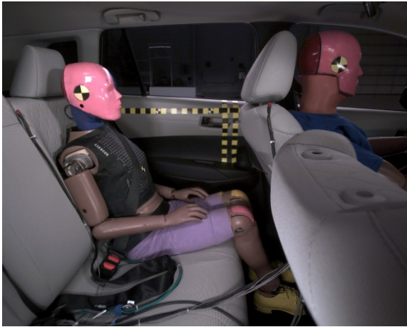
Figure 3a. Lines are marked on the interior of the door at the rearmost point of the front seatback and 50 mm behind that line.
