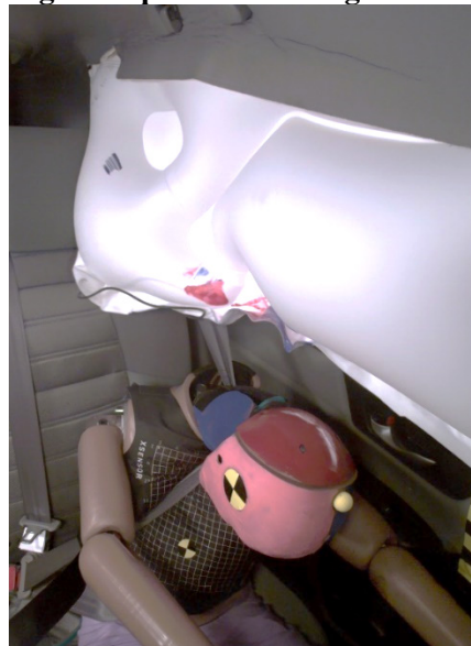
Figure 4 High belt position loading the neck
