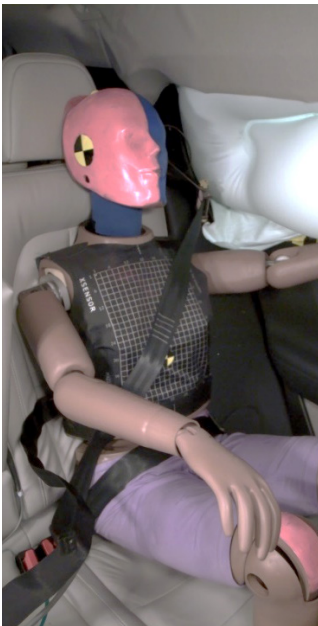
Figure 5a. Stable belt position
