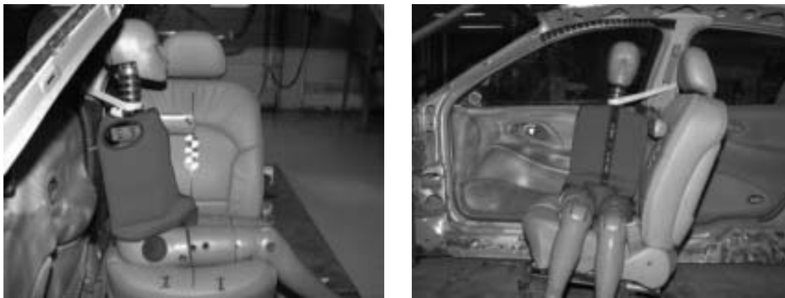
Figure 3.3.5.3.1 Inboard Facing SID-IIs Aligned for Test of Roof-Rail-Mounted Airbag
