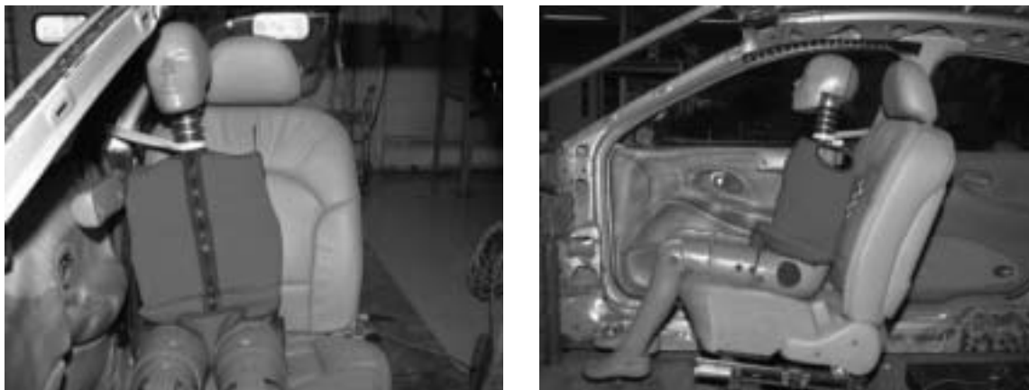
Figure 3.3.5.2.1 Forward Facing SID-IIs Aligned for Test of Roof-Rail-Mounted Airbag
