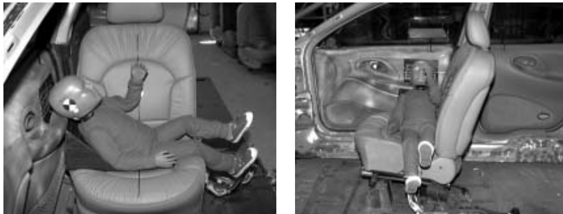
Figure 3.3.4.3.1 Hybrid III 3-Year-Old Child Dummy Lying Across Seat with Head on Door Trim Panel
