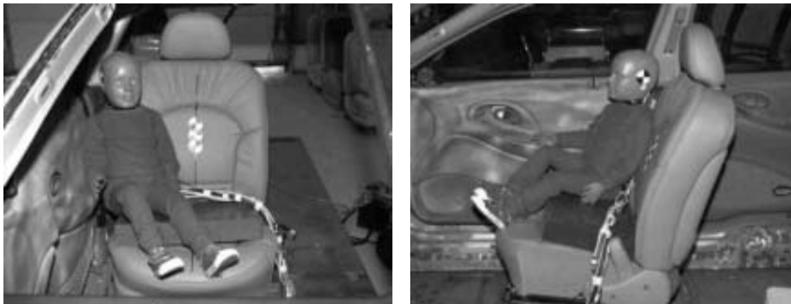
Figure 3.3.3.1.1 Forward Facing Hybrid III 3-year-old Child Dummy on Booster Block Leaning Against Door Trim Panel
