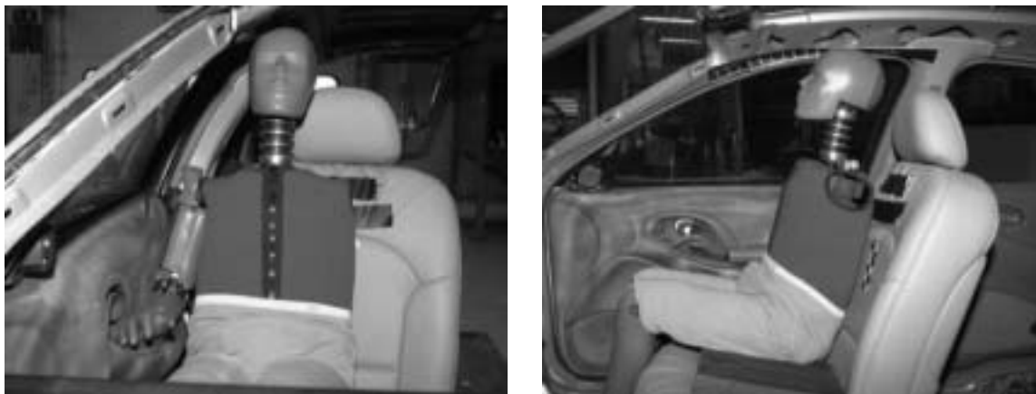
Figure 3.3.3.7.1 SID-IIs with instrumented arm on armrest
