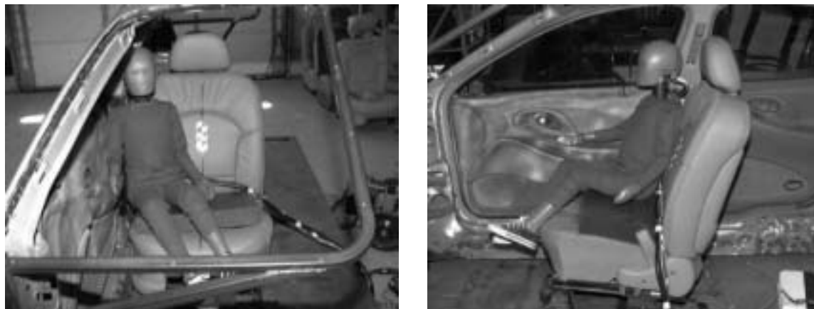
Figure 3.3.3.5.1 Forward Facing Hybrid III 6-Year-Old Child Dummy on Booster Block Leaning Against Door Trim Panel
