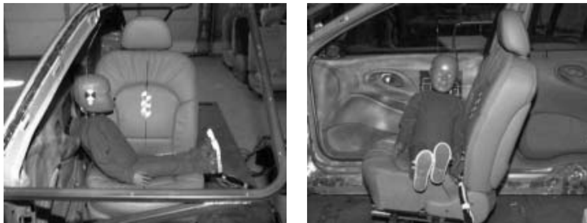
Figure 3.3.4.2.1 Inboard Facing Hybrid III 3-Year-Old Child Dummy Leaning Against Door or Window Glazing
