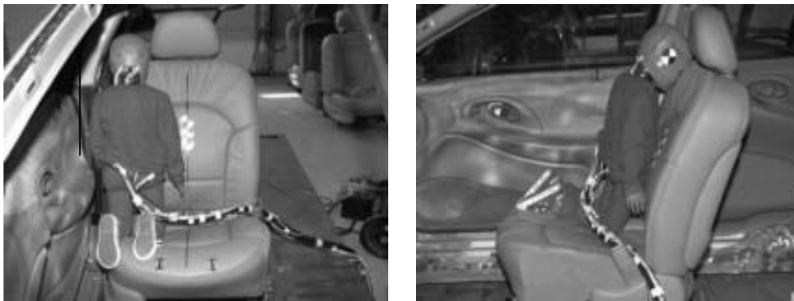
Figure 3.3.3.2.1 Rearward Facing Hybrid III 3-Year-Old Child Dummy Leaning Against Door
