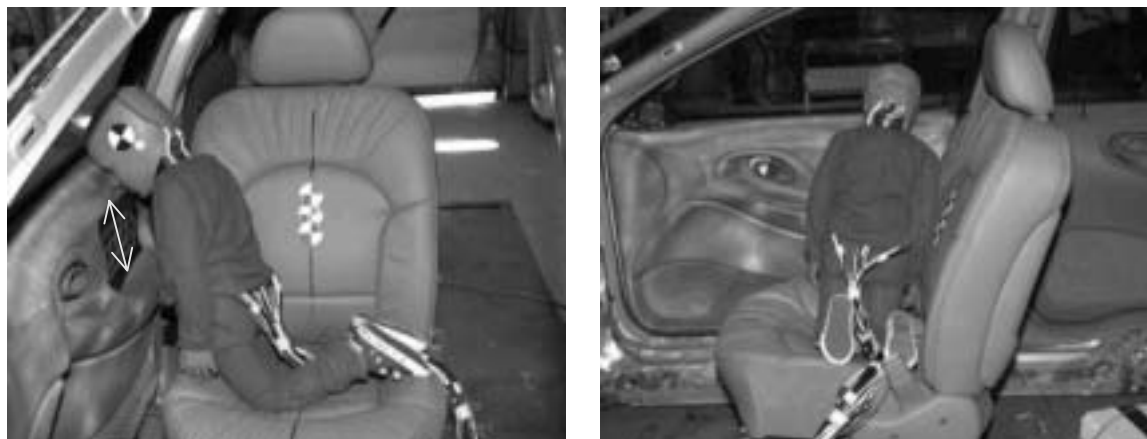
Figure 3.3.4.1.1 Outboard Facing Hybrid III 3-Year-Old Child Dummy Leaning Against Seat and Door Trim Panel
