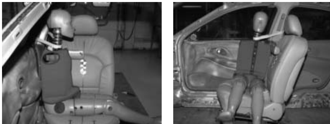
Figure 3.3.3.6.1 Inboard Facing SID-IIs Against Door
