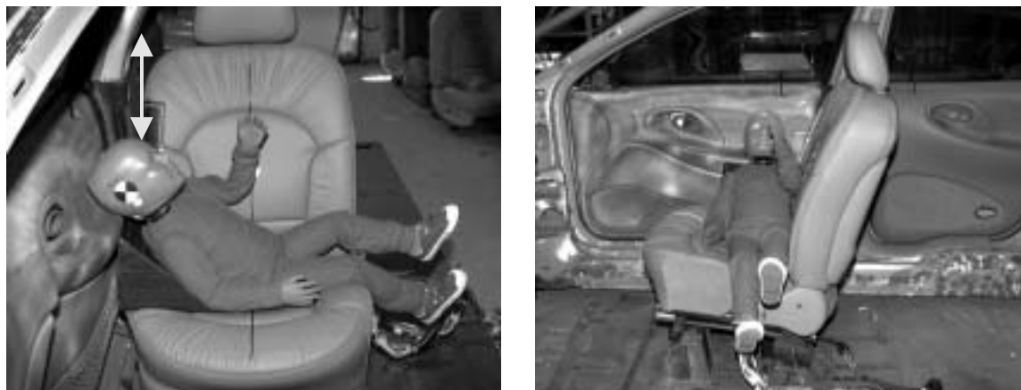
Figure 3.3.3.3.1 Hybrid III 3-Year-Old Child Dummy Lying Across Seat with Head on Door Trim Panel
