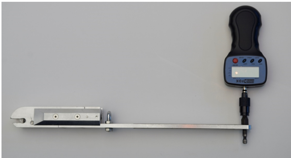
Figure 8. Clearance angle tool with force gauge connected in pull mode.
