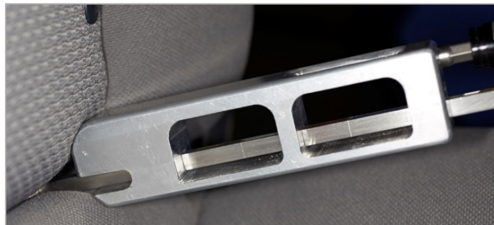
Figure 3. Initial position of force tool slider, with seat cushion just touching top and bottom of front surface of force tool slider.
