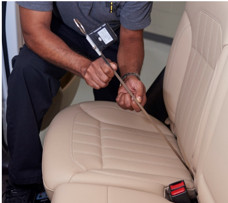
Figure 4. Guide rod rotated upward to the maximum angle until it interacts with the seat cushion or other trim.
