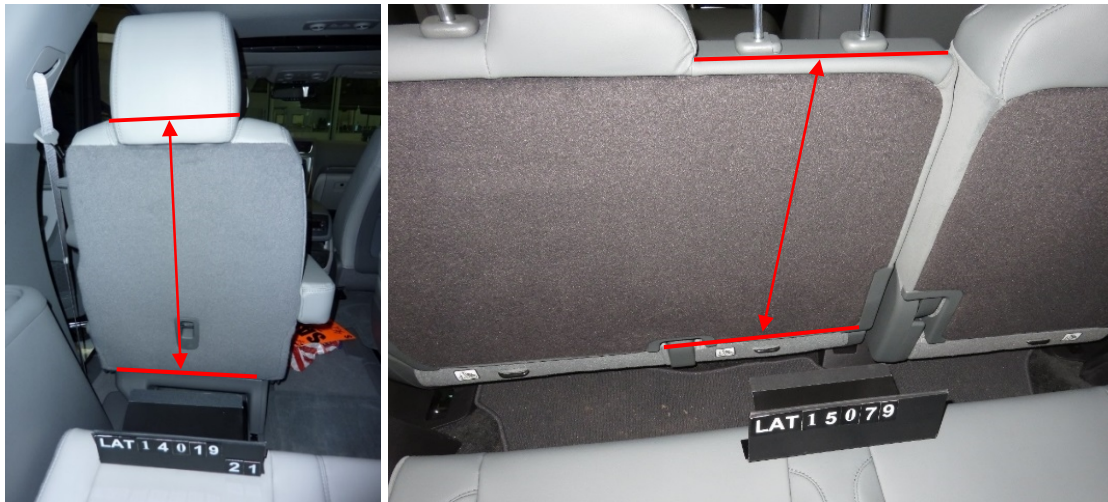
Figure 10. Seatback length, measured on rear of seatback between top- and bottom-most points of seatback.
