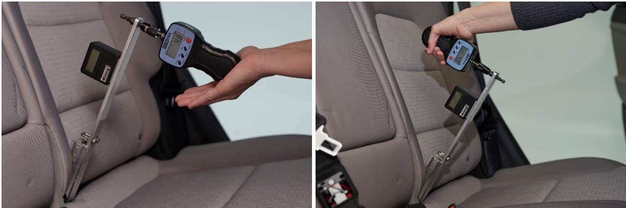
Figure 9. Measuring lower anchor clearance angle in push (left) and pull (right) mode.
