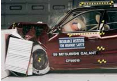
1999 Galant: Structure improved dramatically Overall frontal rating: ACCEPTABLE
