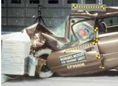
1995 Galant: Occupant compartment virtually collapsed Overall frontal rating: POOR
