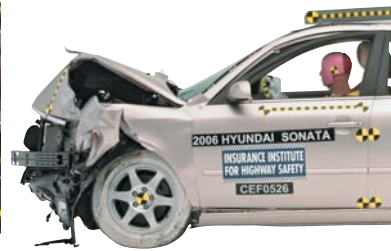
2006 Sonata: Dramatic structural improvement; space around driver dummy maintained
